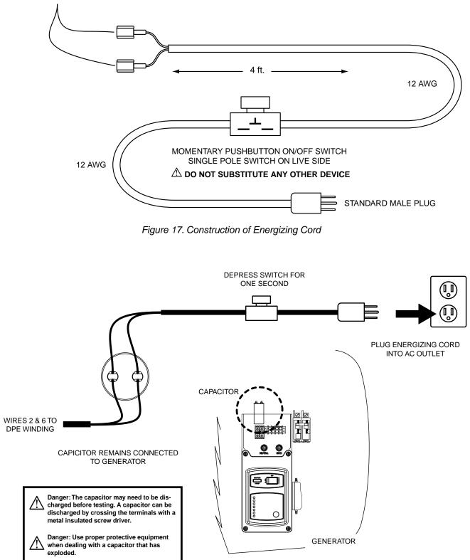
Figure 18. Energizing Cord Connection
